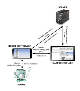
Figure 2. The robot system.
